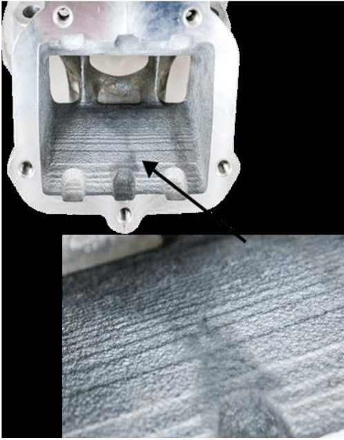
Single Core Cylinder: linear structured cast finish surface
